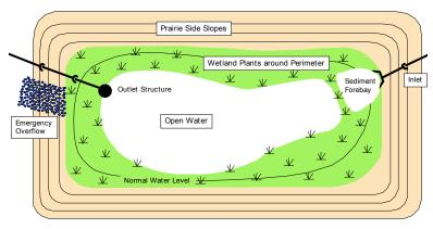
The detention pond's depth influences its water quality. Generally, detention ponds should be deep enough to maintain open water areas and limit sediment resuspension by current, wind, or waves. Typically, the average depth should be at least 4-5 feet and maximum depth at least 8 feet. If you want fish to survive through the winter, it is generally recommended that at least 25% of the pond be at least 10-12 feet deep.
